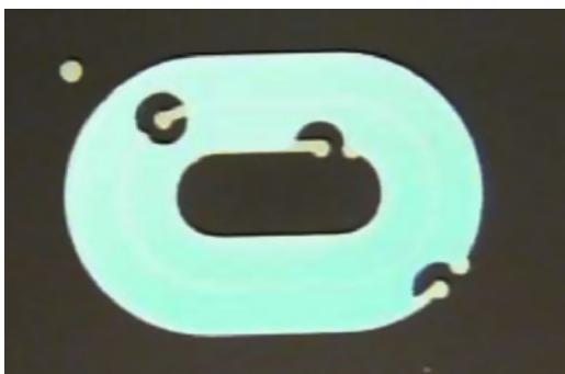
Fig. 5. Highlight of a transformer winding after applying a low-permeability dielectric.
