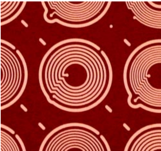
Fig. 1. Close up of 0.006-in. wide conductor pattern printed on a sheet of ferrite tape.
