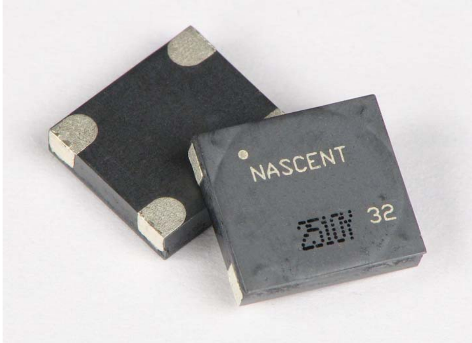
Figure 2: Nascent Technology Flyback transformer D50E
